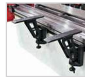
Premium front sheet supports fully adjustable on the linear rails
