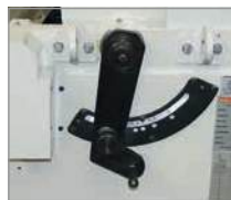
Rapid Blade Adjustment for Material Thickness
