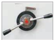
Rapid blade clearance adjustment
