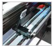
Flip up type back gauge micro adjustment fingers
