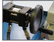
Hydraulic Vice with Pressure Regulator
