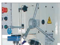
Adjustable Accurate Depth Setting with Auto Feed
