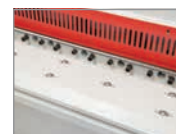
Material Transfer Balls on Table
