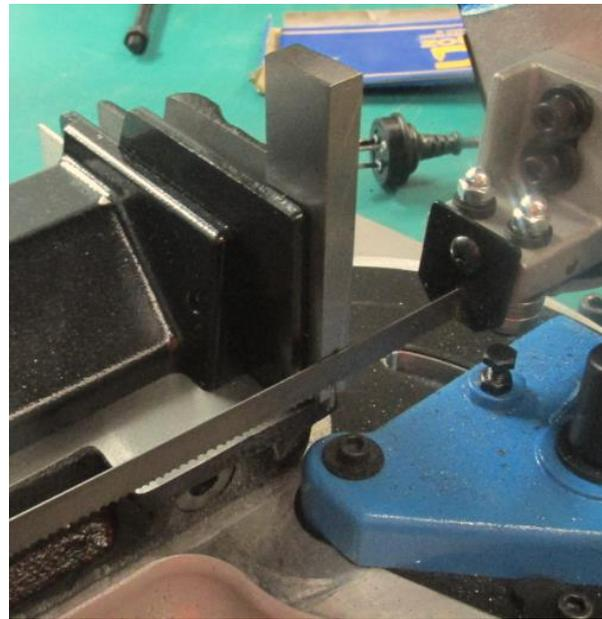
If it does FALL "Square", then the following adjustment is not needed and "other problems" will be the cause such as blade not square to cut fall (Adjust blade guide blocks) or blade faulty ( maybe teeth "Set" worn off one side of the blade )
