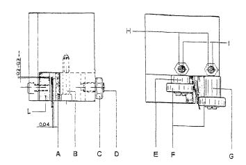
In case the blade needs to be replaced, make sure to always install 0.9 mm thick blades for which the blade guide pads have been adjusted. In the case of toothed blades with different thicknesses adjustment should be carried out as follows:
