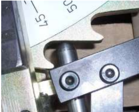
Anti-springback lever engaged
