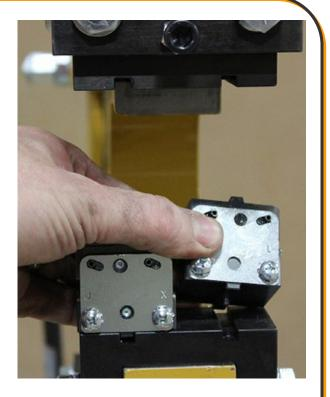
In this view it shows the jaws installed for stretching. Note that the markings "U" are now pointing together, This is the reversing of the jaws from shrinking.
