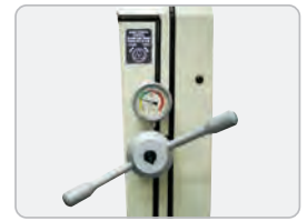
Blade Tension Dial with Gauge BS-461AS
