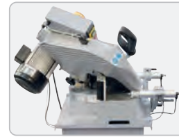
Compound Cut at 45 Degrees Left View
