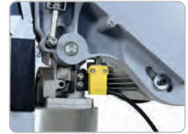
Material Clamp Switch
