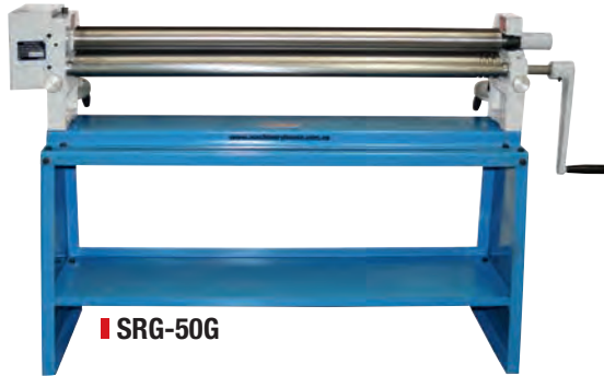
3:1 Reduction Gear Drive SRG-50G
