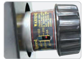
Variable Blade Speed Control BS-10LS
