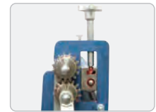
Roll Drive & Adjustment 2.5X50
