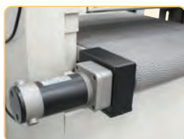
Conveyor Feed Motor
