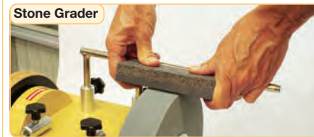
Changes the grains on the grinding wheel for fine abrasion.
