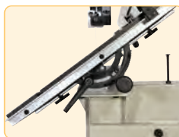
Cast Iron Table Tilts to 45 Degrees
