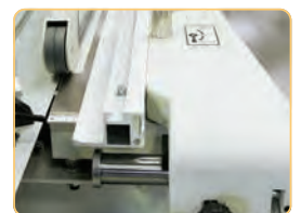
Heavy duty fence with 2 height options
