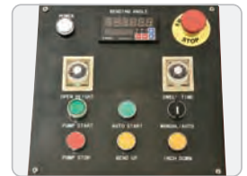
NC Control Panel
