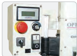
Variable Spindle Speed & Spindle DRO (BF-20LV & MH-28V)
