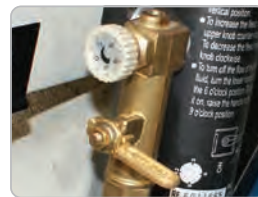
Hydraulic Down Feed Control BS-7L & BS-7DS
