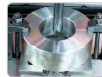
Shown Slotting Keyway with Optional Clamps & Tooling
