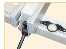
Single Lock Lever on Rip Fence with Magnified Scale
