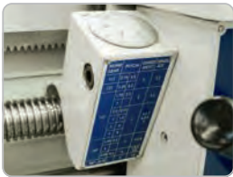
Thread Chasing Dial TM-1740G & TM-1960G
