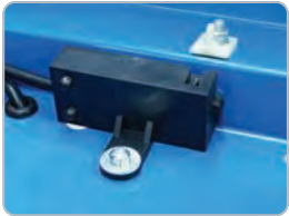
Safety Micro Switch on Pulley Guard
