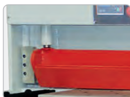
Hydraulic Plate Clamping
