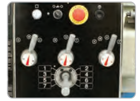
Quick Action Feed Gearbox CL-38A
