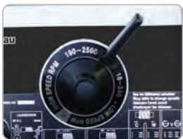
Speed Control Lever DASHIN 2500VS
