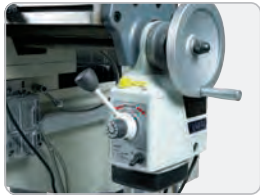
X Axis Power Feed with Rapid HM-51B
