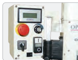
Variable Spindle Speed & Spindle DRO
