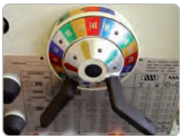
Geometric Progression Speed Selector DASHIN 1550
