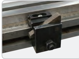
Flip Over Material Stop
