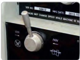
Directional Feed Control Lever AL-320G
