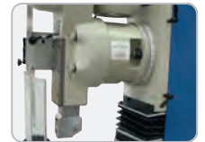
Swivel head tilts left and right 90°
