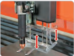
Soft Sense Torch Height Control
