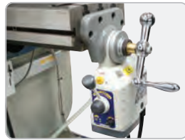
X-Axis Power Feed Unit BM-30A & BM-40V
