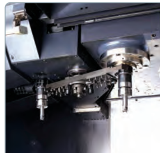
High Speed Arm Type ATC
