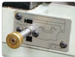
Lubrication Pump DASHIN 1550 & 2500VS
