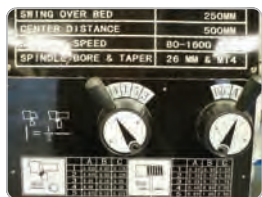
Feed & Threading Gearbox Levers AL-250G
