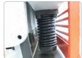
Hydraulic Material Hold Downs
