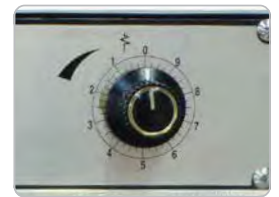
Hydraulic Down Feed Control BS-916A
