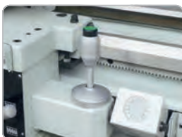
Joystick Feed Control with Rapid
