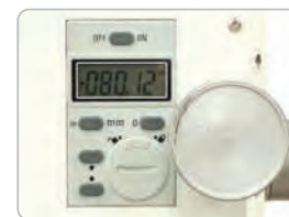
Quill Depth Digital Readout
