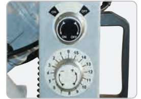
Hydraulic Down Feed Control EB-280DSV
