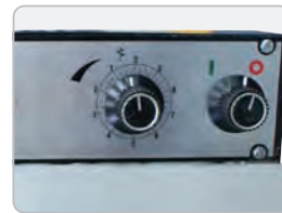
Variable Down Feed Control BS-10LS
