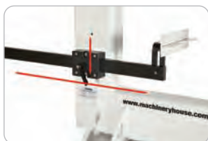
Adjustable Depth Stop Length
