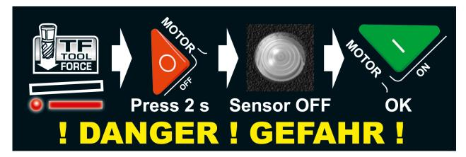
Depending on the version of your core drilling machine it is possible to momentarily deactivate the sensor and its safety function including the automatic MOTOR EMERGENCY STOP.
