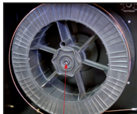
(8) The weight and speed of the wire spool turning creates an inertia that can cause the spool to run on and the wire loop over the side of the spool and tangle. If this happens increase the pressure on the tension spring inside the spool holder assembly using the tension adjustment screw.
