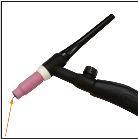
(5) Assemble front end parts of the TIG torch, fitting a sharpened tungsten suitable for DC welding.
