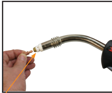
(10) Remove the gas nozzle and contact tip from the front end of the mig torch.
