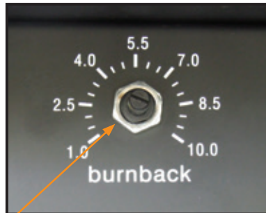
(16) Adjust the burn back control to prevent the wire sticking in the weld pool. Burn back control is located above the wire feed motor
