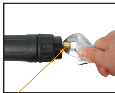
(9) Fully screw down the liner retaining nut and nip it up tight.
