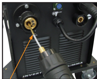
(11) Carefully feed the Polymide liner into the inlet guide tube hole of the torch euro receptacle
