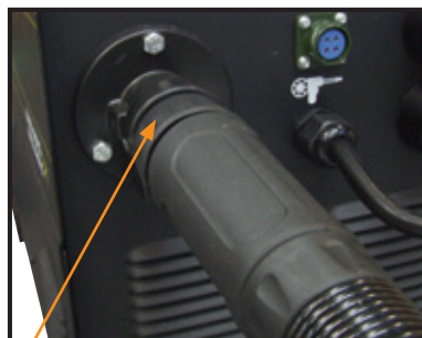
(13) Tighten and secure the torch euro connector to the machine euro receptacle
