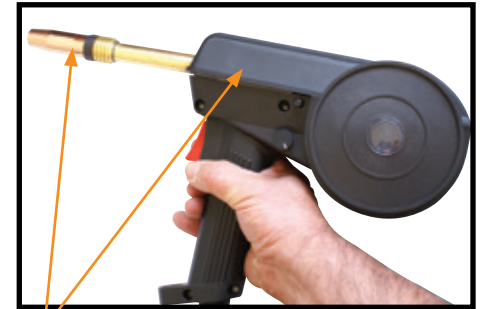
(14) Fit the gas nozzle and close the wire feed spool cover
