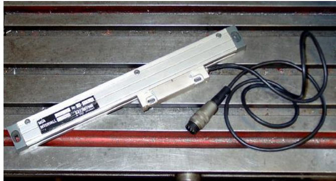
Figure 4.15 - Glass scale encoder (awaiting installation)
