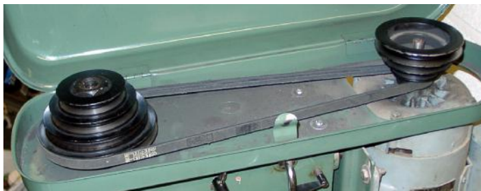
Figure 5.15 - Pulley spindle drive
