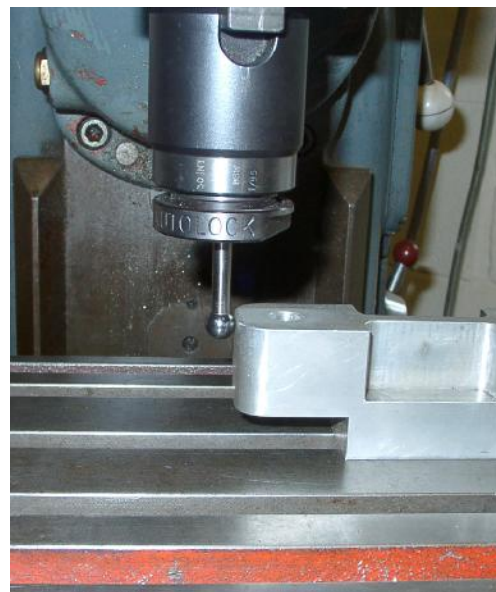
Figure 7.12 - Edge-finder in use on a mill
