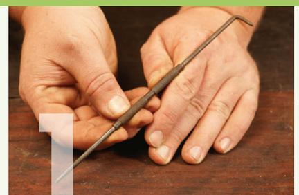
A scriber is the first place to start because it is used to make accurate marks or scratches on metal. While there is nothing wrong with using a pencil or marker pen for basic marking out, if you want accuracy better than plus or minus a millimetre a scriber is the tool to use. This scriber has a straight end for general marking and a bent end for access in restricted spaces. Scribes are sharpened to a fine, sharp point on a bench grinder.
