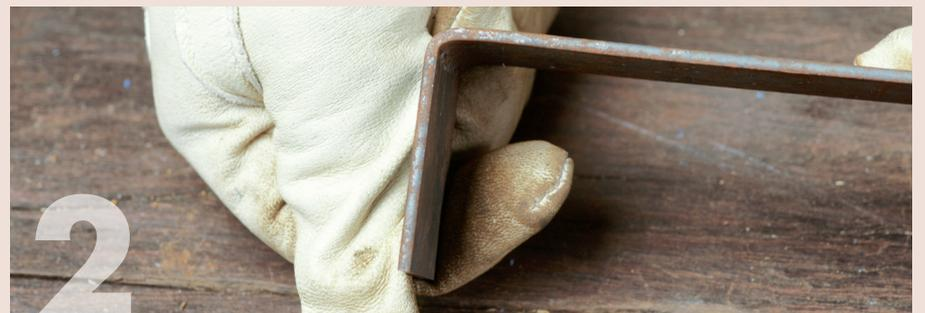
The finished bend should have a nice sharp corner, without any cracks along the outside. If you attempt to bend too thick a section, it will require considerable force, and cracks will form along the outside of the corner.
