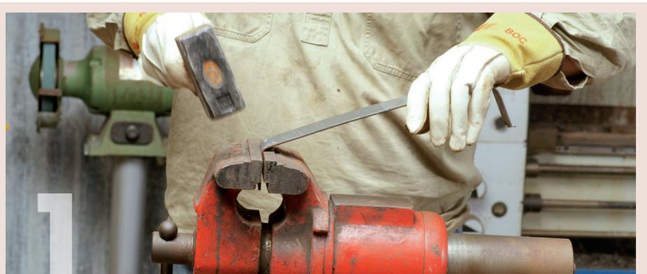
Flat bar can often be bent in the bench vice by clamping firmly, and then striking the bend with a hammer as the steel is pulled over with the other hand.
