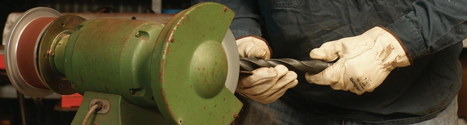
*The bench grinder is capable of more work than simply grinding and can be fitted with a range of accessories for polishing and cleaning metal.*
