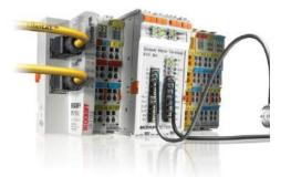
The I/O signals are wired in a decentralised way to fieldbus devices or centrally to the controller. The Beckhoff Bus Terminal ensures that control cabinets and terminal boxes are constructed more economically.
