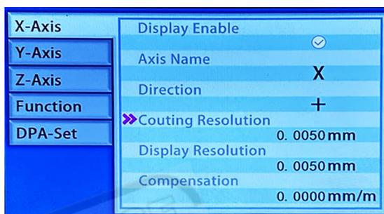
**NOTE: The Display and Counting Resolution should be the same. The compensation field should be left at 0.000 for now. The field is only used when a fault in the “ways “ of the machine is found and this field may be used to correct it.**
