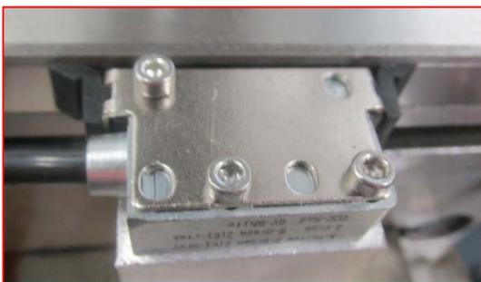
To protect the cable into the head a saddle supplied must be fitted as shown or similar position to all heads. ("Y" Axis Shown)
