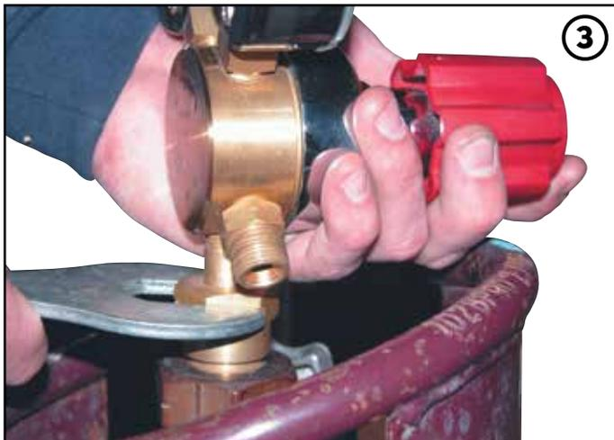
**3 - 3a.** Attach regulators to respective cylinders tighten using appropriate spanner supplied (note: black cylinder for oxygen and maroon cylinder for acetylene)
