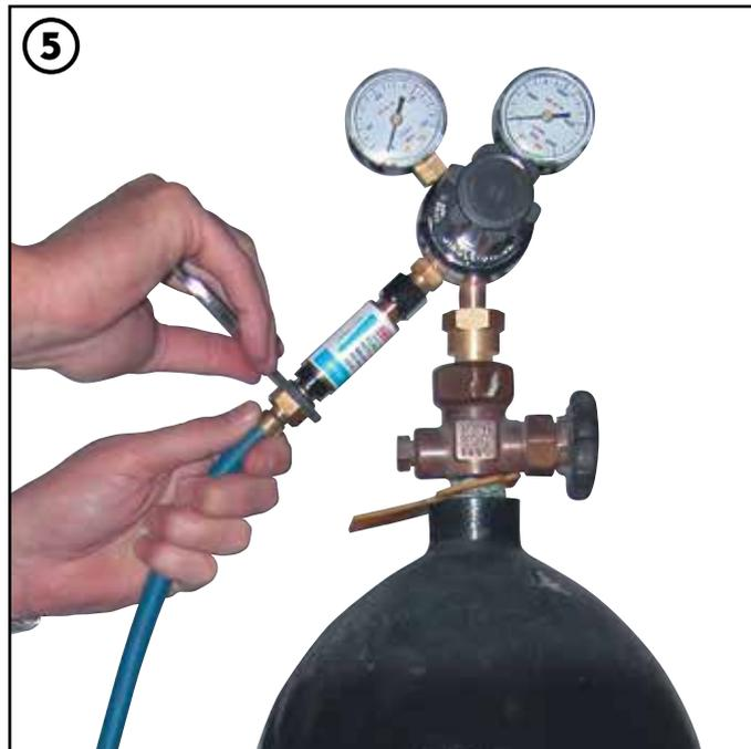
5. Attach gas hoses to flash arrester on regulators using appropriate spanner. **Note: These are colour coded and thread orientated**
