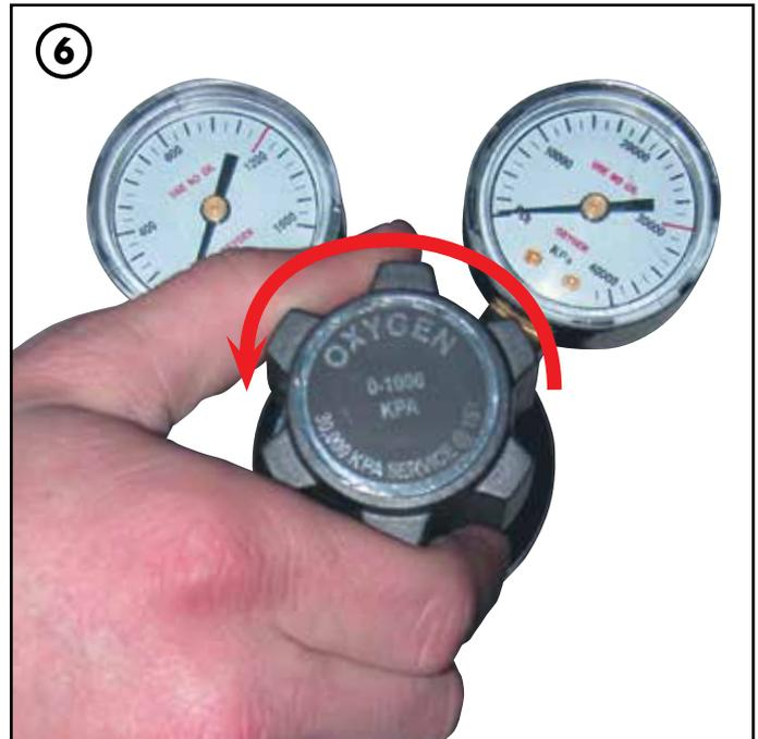
6. Before opening cylinder valves with regulators attached, **ENSURE** that regulator control knobs are fully wound in the **ANTI-CLOCKWISE** position.
