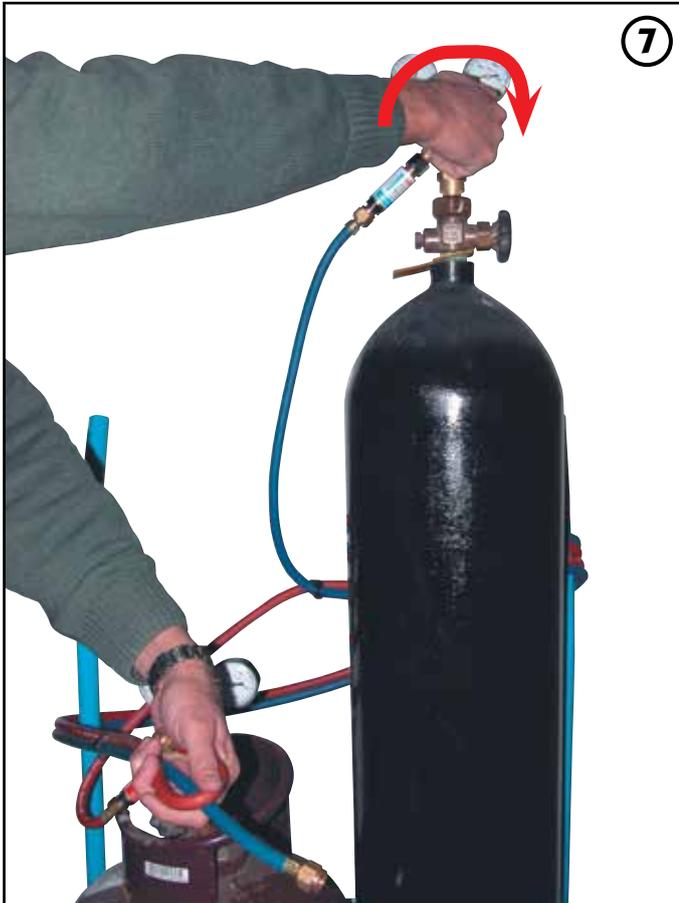
7. Holding the gas hose away from body and any ignition source, slowly turn **CLOCK WISE** the oxygen regulator control knob to achieve a small gas flow to purge any foreign material from tubing. When hose and regulators have been cleared return regulator control knob to the fully **ANTI CLOCK WISE** position. Repeat procedure for the acetylene fuel gas regulator and tubing.
