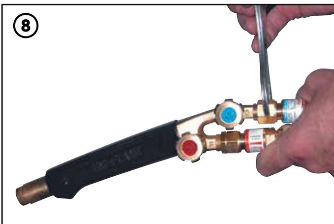
8. Attach **IBEDA** (AS4603) flash arrestors to blowpipe matching the respective colours and threads. Then attach the gas hose, which are colour coded and also thread oriented.
