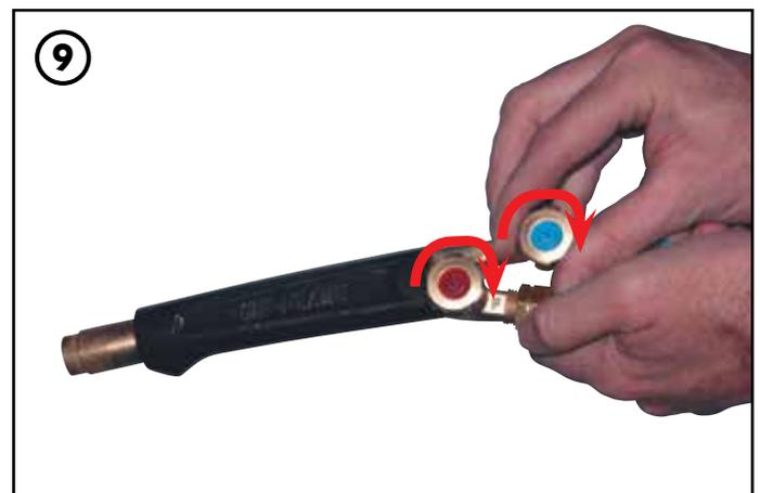
9. Ensure that both blowpipe control valves are closed, open fuel gas cylinder control valve and **CHECK FOR LEAKS**. Then close the fuel gas cylinder control valve and open the blowpipe fuel control valve until both needles on the fuel gauge regulator read zero. Repeat this procedure for the oxygen gas.
