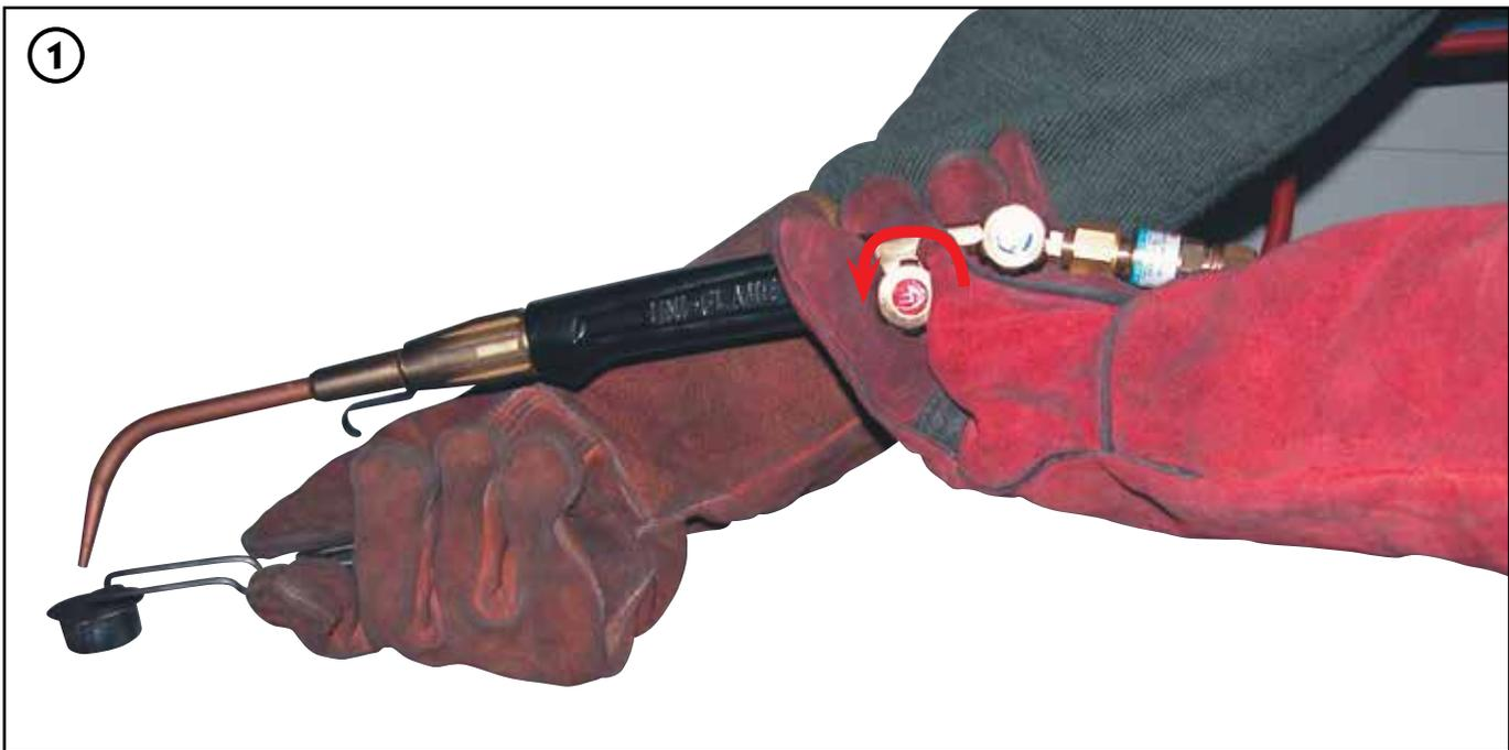
3. Open blowpipe oxygen control valve until a neutral flame is produced.
