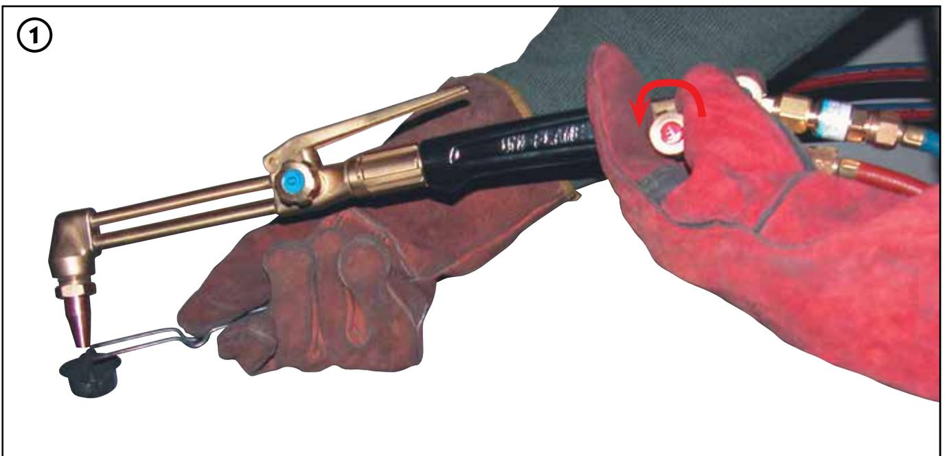
4. Open the oxygen heating control valve until a neutral flame is obtained with the cutting lever depressed. (Refer to flame adjustment setting chart fig A B C & D.)
