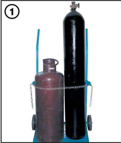
**1.** Secure both oxygen and acetylene cylinders on approved carry stand or trolley. (Not supplied)
