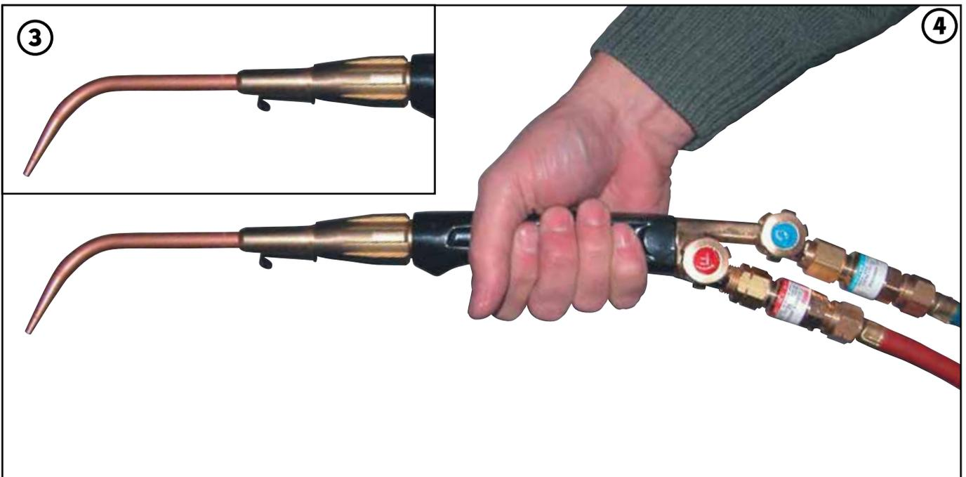
4. Adjust welding tip alignment by loosening mixer to correct the angle of the tip for operators safety and comfort and tighten mixer and **CHECK FOR LEAKS.**
