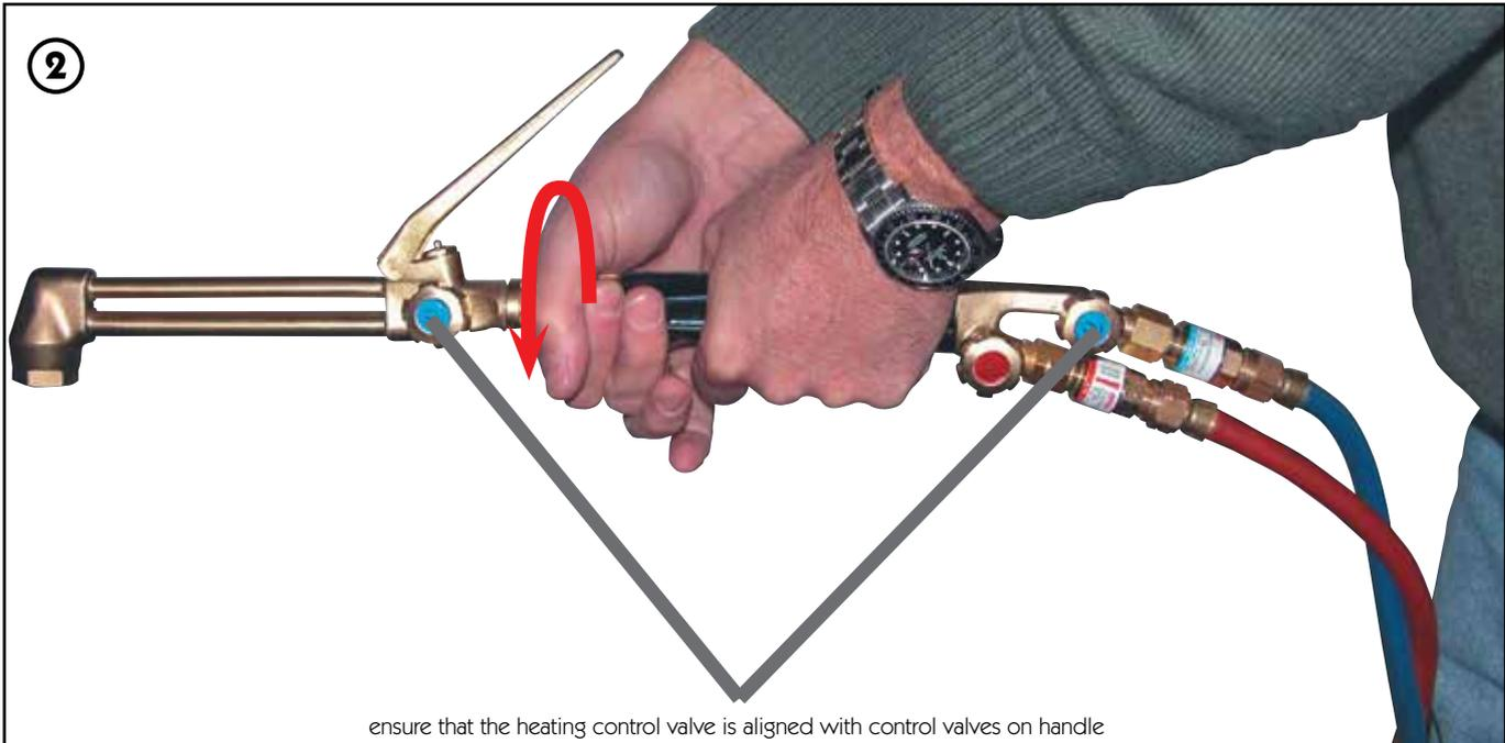
2. Fit the cutting attachment into the blowpipe handle, and ensure that the heating control valve is aligned with control valves on handle **tighten by hand**. Ensure that cutting attachment is secure and **CHECK FOR LEAKS**.
