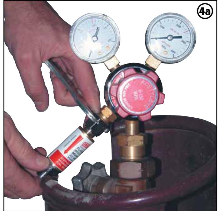
4. Connect approved **IBEDA** flash arrestors (AS4603 supplied) and tighten with appropriate spanner to regulators.
