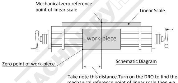
mechanical reference point of linear scale, then we could calculate out the preset zero reference point of work-piece.
