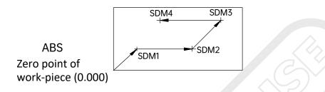
When the DRO is under SDM mode,press SDM button to input the SDM coordinate,or press up and down direction button to switch the coordinate.Traverse the linear scale until the value on each axis become 0. At this moment,this point is the machining point.
