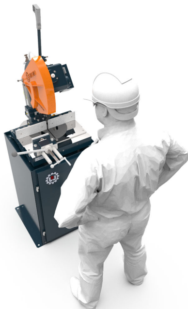
Figure 5. Correct Position for Operating Saw Unit
