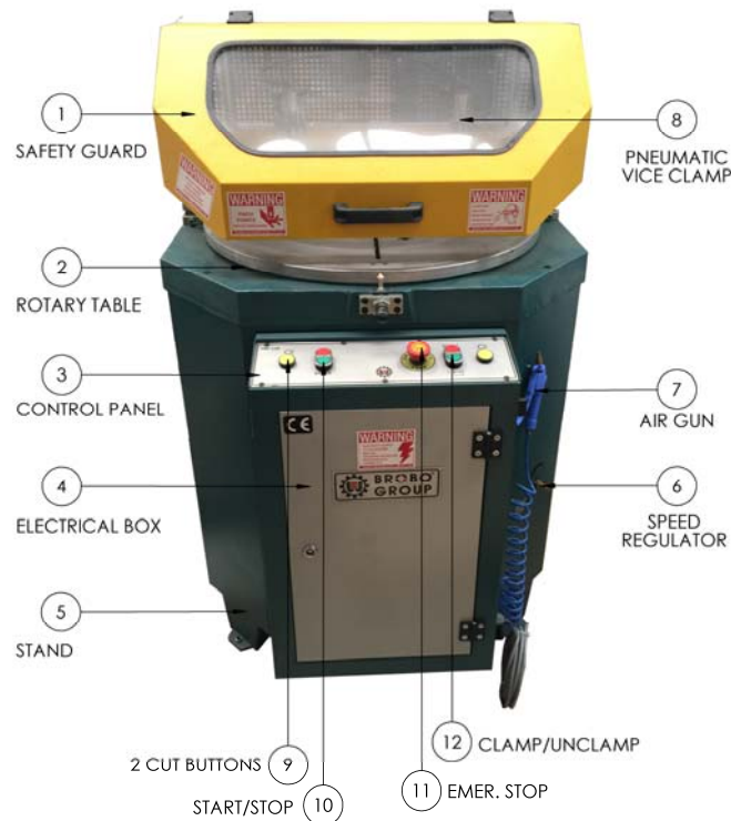
Figure 4. Up Cut Saw Main Components
