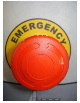
If you see **''Rope Switch Not Set''** message on the screen you need to check whether rope switch is set. For safety you need to set it up. Machine will work after you set rope switch. When the rope switch is set the open contact will close and message will disappear.
