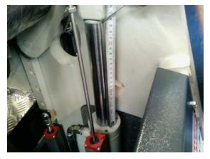
This reference value is entered to the parameter page after distance is measured while Y axis is at top position and touches to the top roll. Each time REFERENCE is done Y axis value is assigned like this automaticaly..
