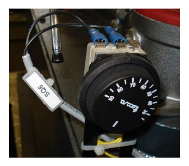
\*\*\* Thermostat which shows the temperature of hydraulic oil is located on oil tank. First you need to check if the temperature control setting is right.
