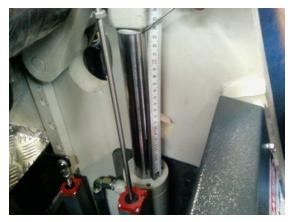
For Y axis, when left cylinder is put completely up and touches top cylinder; calculating opening length with measuring tool, you can find REFERENCE value and write on parameters page. Whenever you do REFERENCE, this REFERENCE value will be assigned automatically for Y axis. This value is also written for Max. limit parameter.
