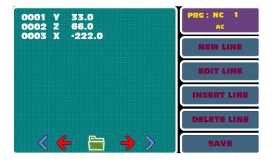
Position values which is more than min & max values of the axis shouldnt be written during recording a program because that will makes axis to go beyond its max value so it will stop the program
