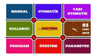
NC Unit provides you to control an axis on manuel, automatic and semi automatic mode Axis can be moved by control buttons .NC Unit has 500 program storage capacity and 200 line can be saved on each program and program storage may improved up to 10.000 program with USB flas memory disc .If you press the company logo at the middle of main page screen settings and company contact informations comes up and if you press onto screen then you transfered to main page again
