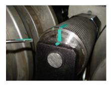
To calibrate 'X'' rotation axis, firstly you need to calculate the circle area of top roll (cylinder). It is calculated by multiplying **Pi number** (3.14) by diameter of top roll (cylinder).
