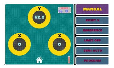
On Manual mode axis can be moved manualy with the buttons and animation of the movements can be seen on the screen ,roll directions , encoder reading directions can be checked
