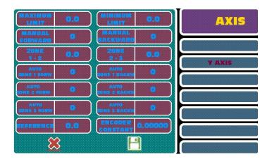
In this page there are position sensitivity settings of axes. *NC* unit calculates the parameters automatically and these parameters become active. Also *NC* unit updates these parameters automatically.
