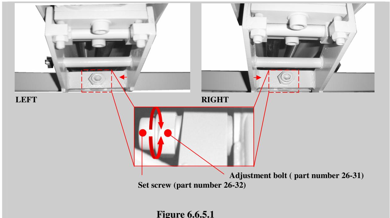
In case of existing a difference on one of the sides (left or right), loosen the set screw and adjust the parallelism by turning the back-gauge bolt (see **Figure 6.6.5.1**). Tighten the set screw.
