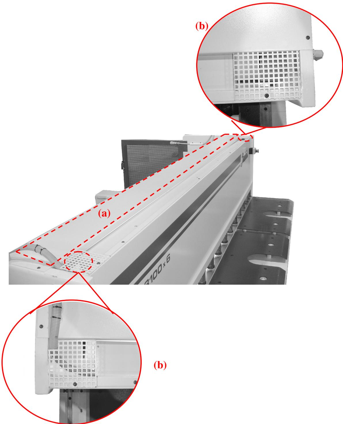
The plate (a) and grid (b) are used to protect the operator from accidental contact while the cutting beam is moving upward and downward
