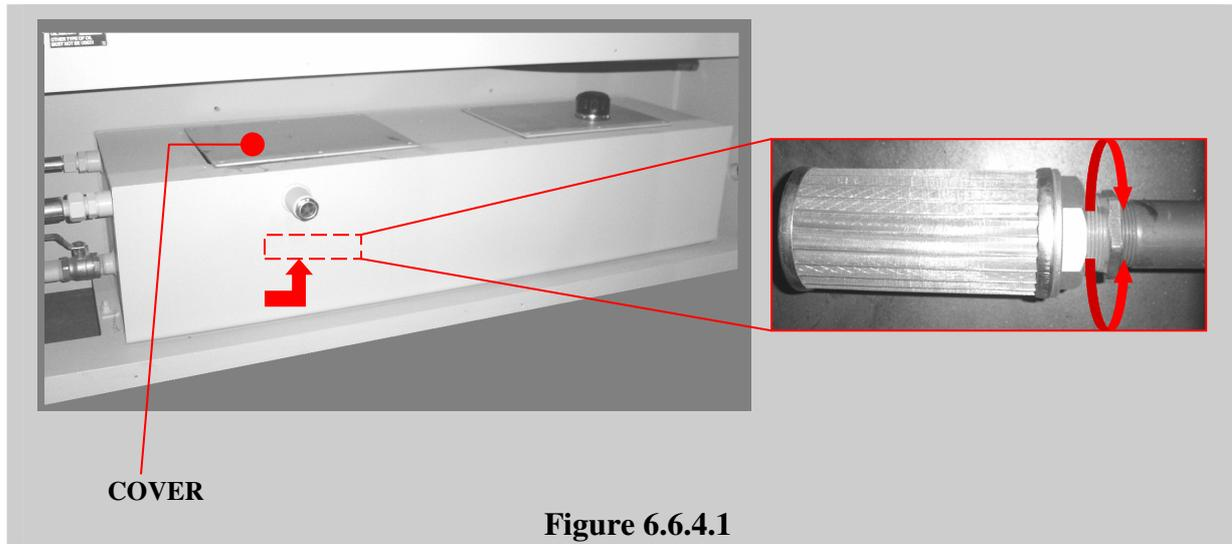
1. Remove the cover on the oil tank after loosening and pulling out the screws.
