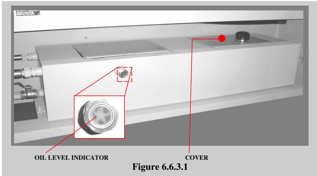
1. Remove the oil tank cover after pulling out the screws.
