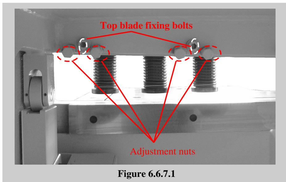
**g)** Repeat the procedure in (f) for all fine adjusting bolts alongside the blade length from left to right.
