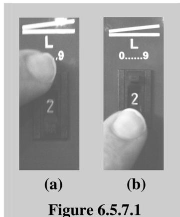
Use **the stroke timer** on the control panel to adjust the cutting length.(Between 0-9, while 9 is the full length).
