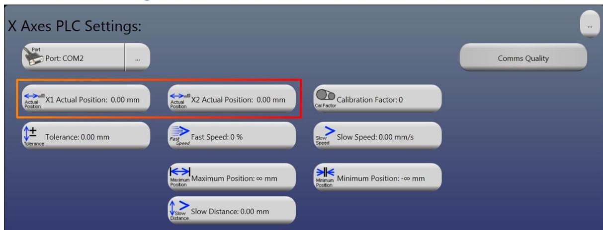
Both sides of an axis share settings when connected to the PLC. The actual positions may be different.
