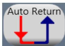
Press on the AUTO Return button so the 2 arrows are **not** connected. Press start and wait for the machine to position. Place the test piece on the Die.
