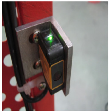
Receiver - Green light on. Indicates power is on but not aligned.
