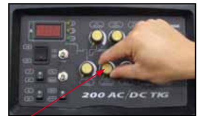
(4) Set the Pulse Frequency at 2 Hz
