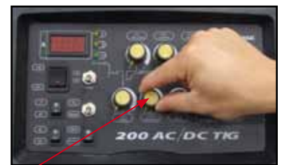
(4) Set the Pulse Frequency at 2 Hz
