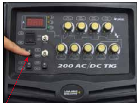
(10) Select 2T or 4T trigger function as required
