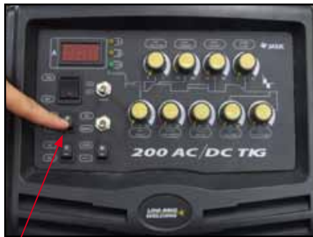
(2) Select 2T or 4T trigger function as required
