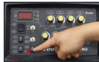
(6) Set the Pulse Selector switch to Pulse
