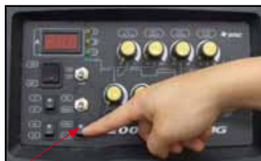
(6) Set the Pulse Selector switch to Pulse
