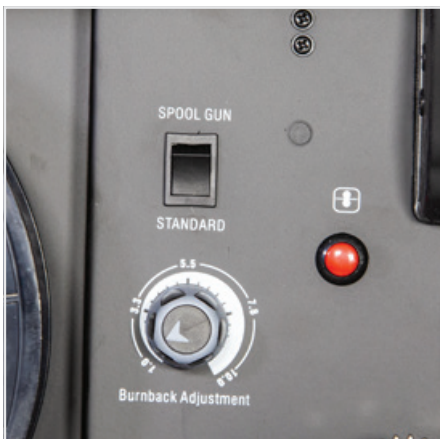
(2) Set Spool Gun / Standard selector to Spool Gun .
