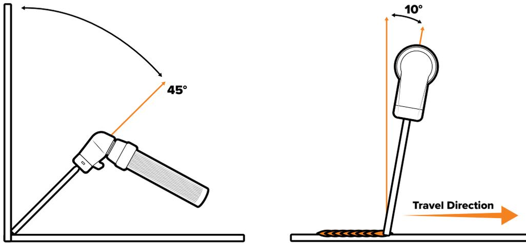
As you weld, keep your arc length short. A good rule of thumb is that your arc length shouldn't be longer than your electrode diameter. If you're using a 2.6mm electrode, your arc length shouldn't be longer than 3mm. However, you don't want to be so close that your electrode is touching the metal, as it will stick. If you pull away too far, your arc will become unstable, you'll produce more spatter, which will fly everywhere, and it'll become hard to keep the arc lit.
