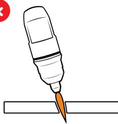
Torch angled to the material. Unequal bevel, one side may be excessively bevelled.
