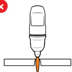
Torch height too low. Reverse bevel. The tip may contact the work and short out or damage the tip.
