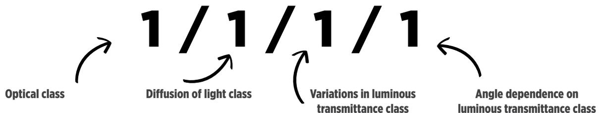
**Optical class:** how distorted is the image through the lens? If you look through the lens and it's like looking through rippled water, then it's not a good helmet. The image should be clear and crisp to obtain a 1 rating.
