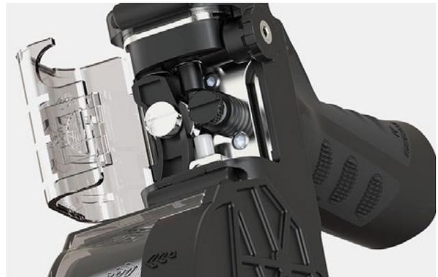
As well as your standard MIG torches, you can also get an aluminium specific torch, called a 'spool gun'. Spool guns are set up slightly differently than the MIG torches, as the wire spool is not connected in the machine but in the gun itself. The spool holder can only hold 1kg rolls, so if you're doing a lot of aluminium welding, it'll run out faster than in a machine, and the gun is going to fatigue your hands faster.
