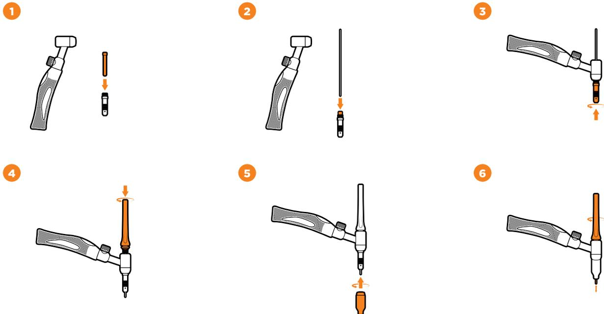
Keep in mind that the tungsten shouldn't stick out further than the inner width of the ceramic cup. For example, a #7 cup is 11mm wide, so the tungsten shouldn't sit further out than 11mm from the top of the cup. It's okay if your tungsten is sticking out too far after you've screwed the back cap on; just unscrew it until the tungsten becomes loose, slide the tungsten back until it's the correct length and then re-screw the back cap until the tungsten is snug again.
