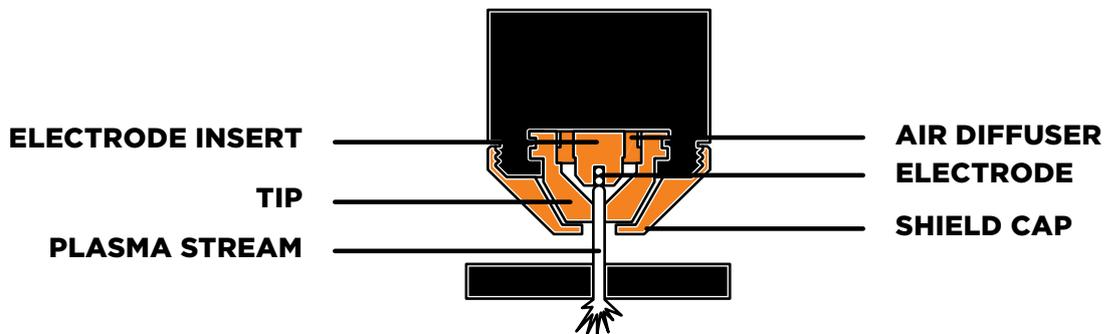
Plasma can cut through anything electrically conductive; steel, stainless steel and aluminium are all fair game. In comparison, oxy cutting will only work on metals that contain iron, as it works through chemical reactions, such as oxidisation (it's like a sped-up version of rusting) instead.
