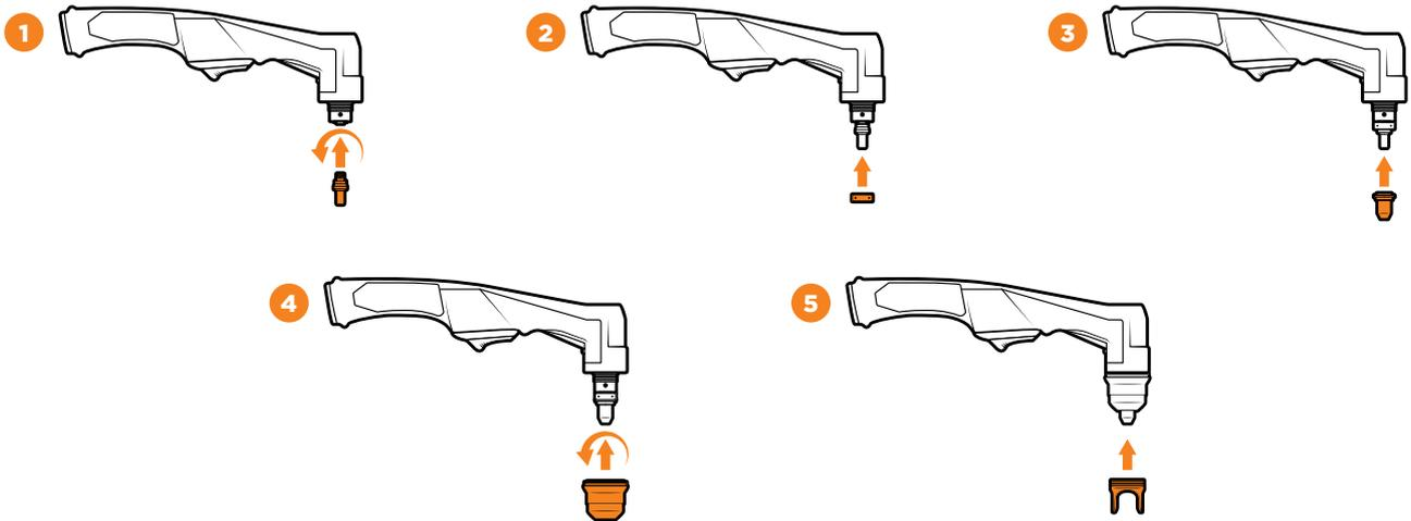
The higher-end torches will also need a cooling tube. The tube sits inside the torch head, and the electrode is screwed on like normal over it.
