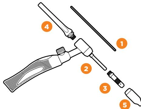
The collet and collet body should match the size of your tungsten (if your tungsten is 2.4mm thick, the borehole in your collet and collet body need to be 2.4mm wide).
