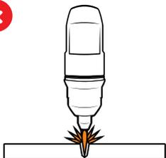
If sparks are spraying up from the workpiece, you are moving the torch too fast, or you don't have enough amps set.
