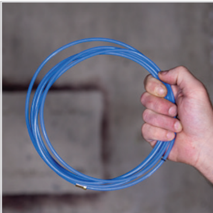
(4) Carefully unravel the new liner
