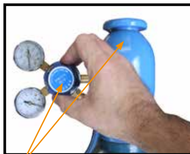
(6) Carefully open the valve of the gas cylinder, set the flow to 6-10 l/min
