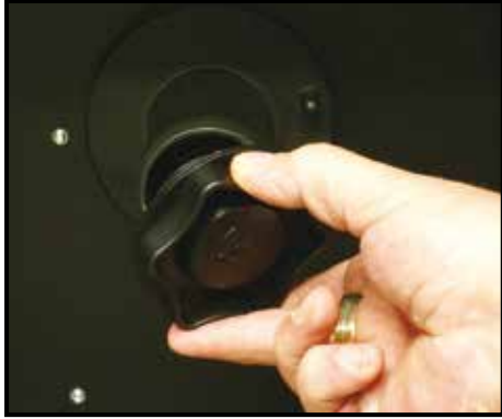
(1) Remove the spool retaining nut.
