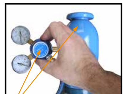
(14) Carefully open the valve of the gas cylinder, set the flow to 6-10 l/min
