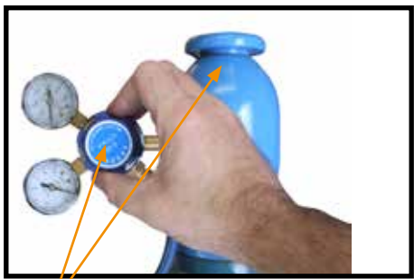
(15) Carefully open the valve of the gas cylinder, set the flow to 6-10 l/min
