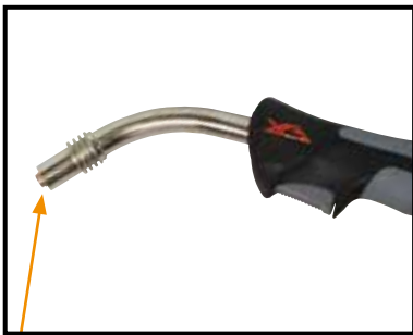
(1) Remove mig torch front end parts
