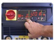
The Ergonomic and Auto Learning System is used in the powerful front panel interface where welding mode selection, program selection, adjustments and special settings coexist in a rugged panel, whereby with a simple touch the user can instantly see the results they have selected.
