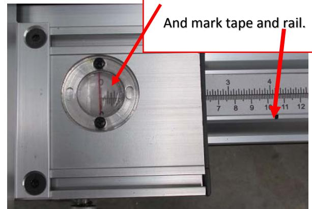
Start peeling the backing tape off the new tape and position the tape on the rail, lining up the black marker lines as you go, then if all Ok, peel the rest of the backing paper off as you put the rest of the tape into the groove. Press the tape down firmly along its length.
