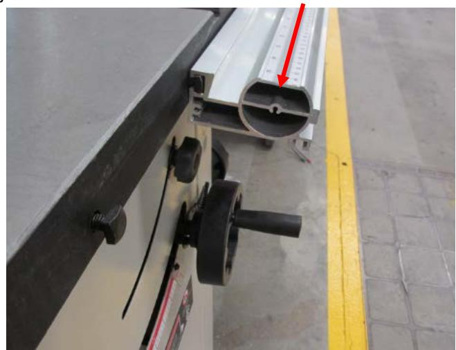
**For set up #2** Align each rail so it is in front of the left edge of the main cast table about 8 to 10mm
