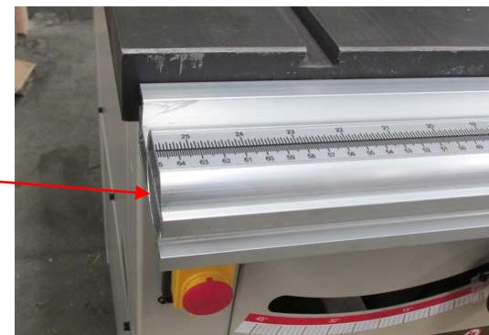
Find the Rip fence assembly complete with the Side extension plate.
