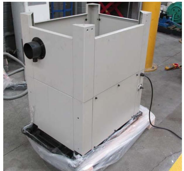
Fit the Rear panel "E" with the dust extraction cufe fitted to the rear of the machine on the side marked "E"
