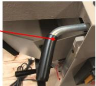
When this is set, the Infeed table must be checked to ensure its top stop aligns the infeed table with the outfeed table.
