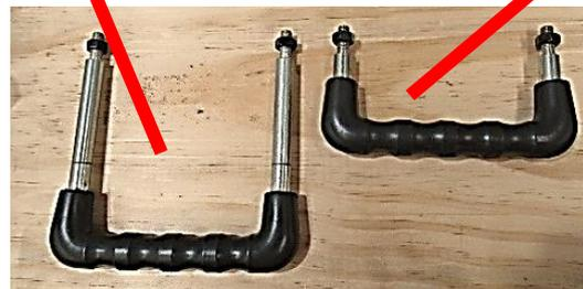
Please note. as described in the current manual supplied the adjustment of the table for setting the knife states to unlock and adjust the 2 positioning studs.. These do not get adjusted and are only for adjusting the table/s parallel to the spindle blades on resetting of the spindle.
