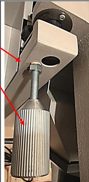
When this is set, the **Infeed table** must be checked to ensure its top stop aligns the infeed table with the outfeed table.
